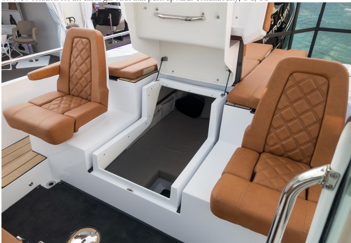
10. New solution for aft cabin gas strut that push upwards continuously, OC/TT
